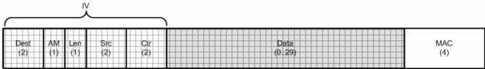
(a) TinySec-AE packet format
