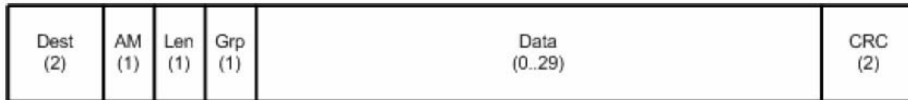
(c) TinyOS packet format
