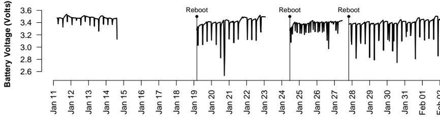
**Fig. 2.** An example of a mote rebooting due to low battery voltage (no watchdog timer in use). The sharp downward spikes correspond to gateway downloads (every six hours). Gaps in the series are periods where the mote was completely inoperative.
