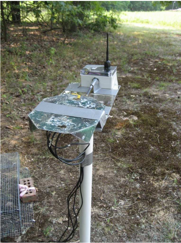
Fig. 1. Environmental monitoring mote deployed in the Jug Bay wetlands sanctuary to monitor soil moisture and soil temperature.
