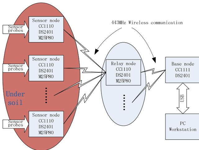
Figure 2. Structural diagram of the proposed soil measuring WSN.
