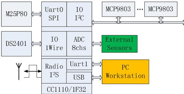
Figure 4. Components and connections of proposed soil-measuring WSN node.
