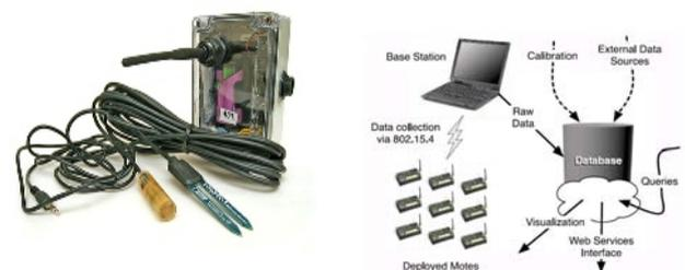
Figure 1. Sensor node and data collection architecture for the Life Under Your Feet project.
