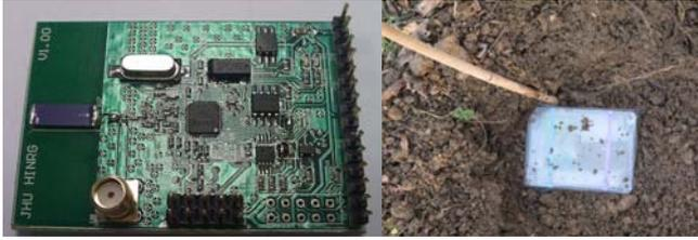
Figure 3. Sensor board of WSN node in the lab. The same node is shown inside a field enclosure before placed below ground for radio communication experiments.
