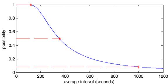
Figure 6. Relationship between the possibility of at least one successful connection a day and the average wake-up interval. In all cases radio on time is fixed to one second.
