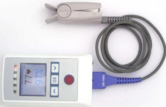
Fig. 2. Medical information tag, or miTag for short, used in MEDiSN [43]. The miTag is a Tmote mini [53] based patient monitor that includes a pulse oximetry sensor with LEDs, buttons and a LCD screen. The miTag is powered using a re-chargeable 1,200 mAh 3.7 V Li-Ion battery and external finger tip sensors are used to make the pulse oximetry measurements.
