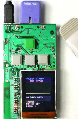
Figure 4: Custom vital sign collecting hardware developed for MEDiSN.
