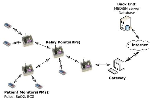
Figure 1: The *MEDiSN* Architecture, including multiple Patient Monitors (PMs) that collect patients' vital signs, Relay Points to forward the data and a gateway to collect individual measurements from PMs and send management commands.
