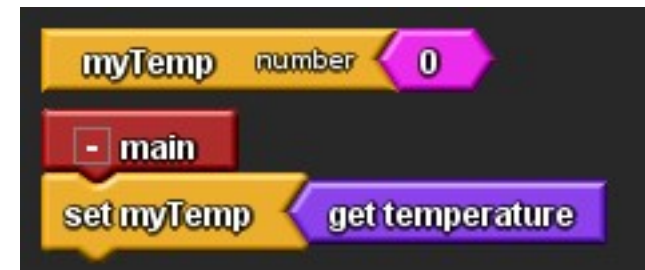
Specialized Block Getting temperature data on a mote
