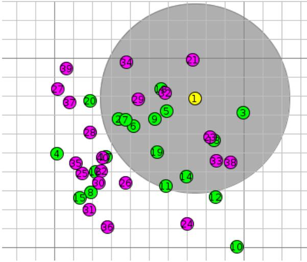
**Figure 2: The simulation topology consists of 40 nodes, 39 sender nodes and one sink. The figure shows a sample topology in which ContikiRPL nodes (lighter nodes) and TinyRPL nodes (darker nodes) coexist. We show the communication range of the sink (node 1).**
