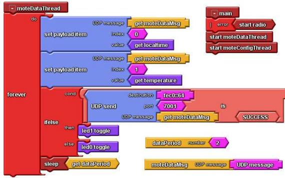
Figure 4: TinyInventor example application, mote code part 1. Contains the main thread and the data thread which periodically samples the motes temperature sensor and sends it to a PC.
