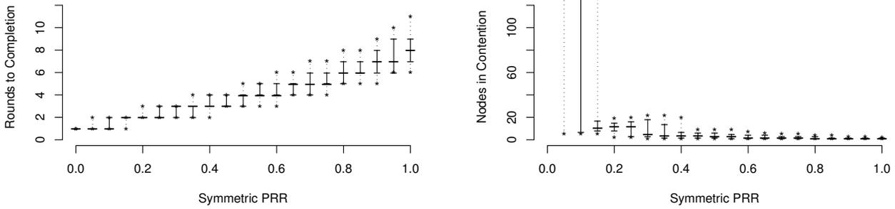
(a) When link quality is poor, negotiation time is low: the receiver stops the process at the first round where no acks are received. (b) “Early stopping” leaves many nodes in contention, as few eliminations occur.
