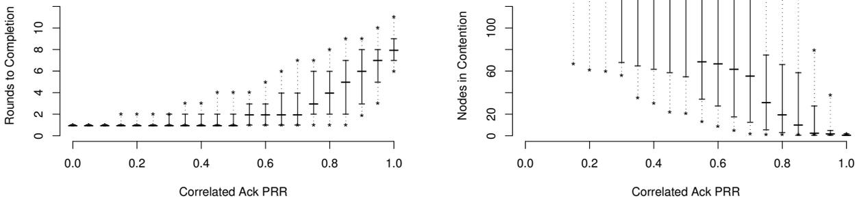
(a) Losing all acks stops negotiation immediately. When ack PRR is low, (b) If acks are not reliable (e.g. due to persistent interference at the receiver), Flip-MAC is not able to effectively reduce the level of contention.
