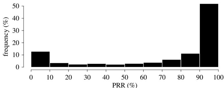
Figure 6. Distribution of packet reception ratios (PRR) across all the links from a 52 node data centre site survey described by Liang *et al.* [18]. A large percentage of the network's links exhibit non-trivial loss rates.
