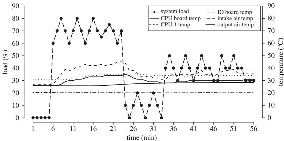
Figure 5. Temperature measured at different locations in and around an HP DL360 server. Also shown is the server's CPU load. Internal sensors reflect the workload of the servers instead of ambient conditions.
