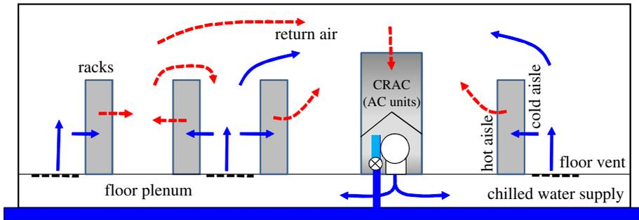
Figure 1. An illustration of an air-cooled data centre on raised floors. Dashed arrows indicate ‘hot’ and solid arrows indicate ‘cool’. (Online version in colour.)
