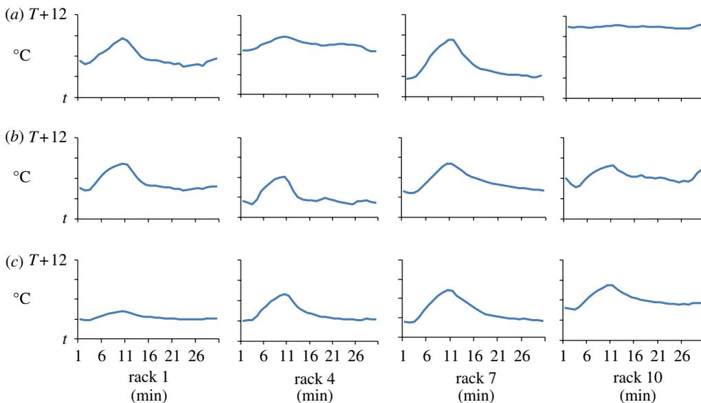
Figure 11. Temperature data from a row of ten racks, labelled from 1 to 10, during a thermal runaway event. Each rack has three sensors at the (a) top, (b) middle and (c) bottom, respectively. Temperature changes depend on locations. (Online version in colour.)
