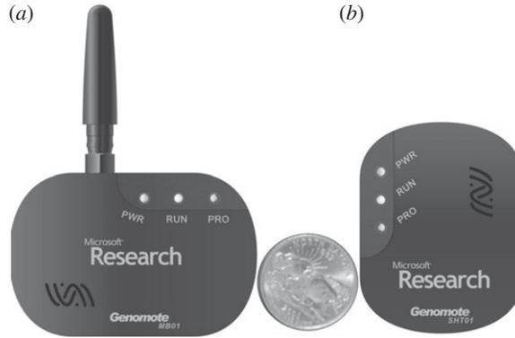
Figure 9. Two types of sensors designed for DC Genome. (a) The wireless node controls (b) several wired nodes to reduce the number of wireless sensors within the same broadcast domain.
