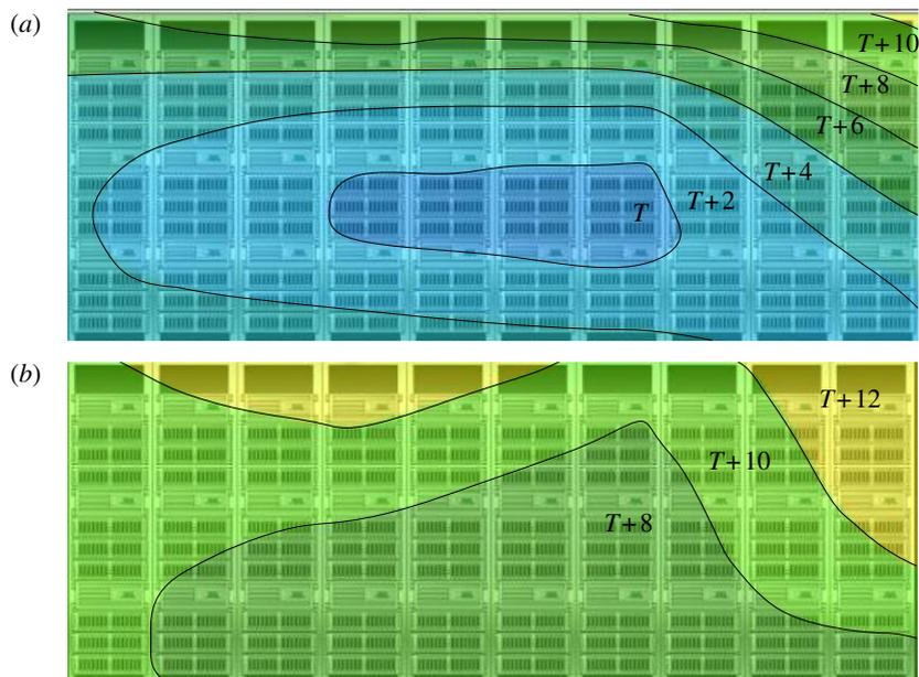
Figure 3. (a) Cold aisle and (b) hot aisle heat maps generated from sensor data. (Online version in colour.)
