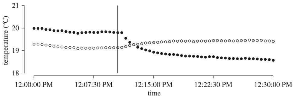
Figure 4. The intake air temperature of the controlled server decreases after the server is shut down, while the temperature of the server below increases. The vertical line indicates the time when the controlled server was shut down. Filled circles, controlled server; open circles, one server below.
