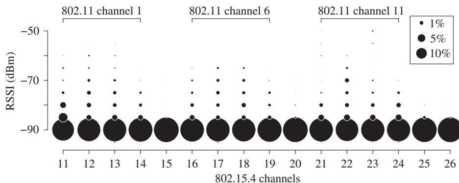
Figure 8. Background noise distribution across all 802.15.4 frequency channels in the 2.4 GHz ISM band. Each of the circumferences is proportional to the occurrence frequency of the corresponding RSSI level. Channels 15, 20, 25 and 26 are relatively quiet compared with other channels.
