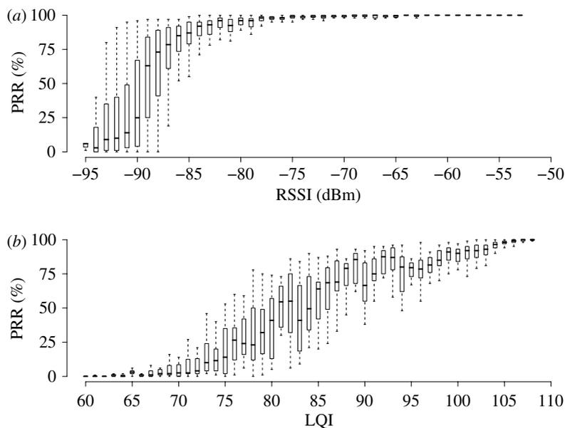
Figure 7. Boxplots of link PRR as a function of (a) received signal strength indication (RSSI) and (b) LQI values from the data centre RF survey in [18]. Boxplots show the sample minimum, first quartile, median, third quartile and sample maximum. Links with  $\text{RSSI} \geq 75$  dBm and  $\text{LQI} > 90$  have persistently low PRR.
